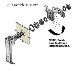
Pawl should be adjusted to GRIP measurement with the door open and the handle in the LATCHED position. Use two wrenches to tighten.
