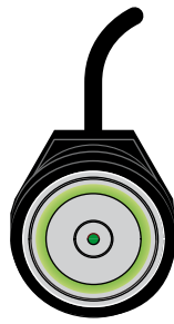
Reader LED turns green (enrolled key)
