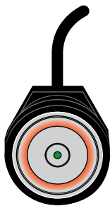
Reader LED turns amber (programming mode)
