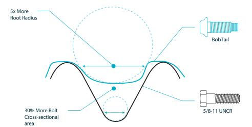
The unique design of our lockbolt pins have shallow locking grooves so they have a larger root radius than conventional nuts and bolts of the same size. This provides 30% more pin cross sectional area and improved notch factor for 5X improvement in bending and tensile fatigue strength.
