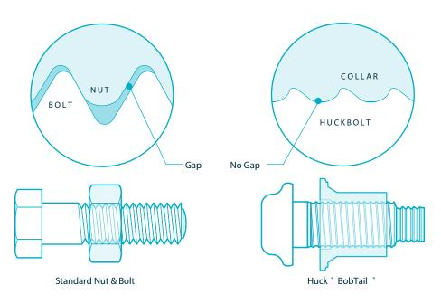
Conventional nut and bolt installations leave gaps between the threads that lead to loosening in high-vibration conditions. HuckBolts use a unique swaged metal collar that is pressed into the steel threads of the pin as part of the direct-tension installation process; thus eliminating these problematic gaps.
