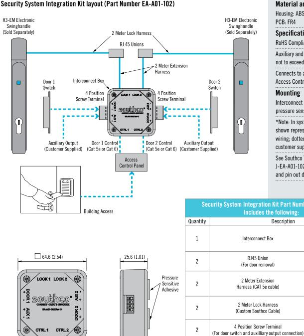
**Material and Finish** Housing: ABS, UL94-5VA PCB: FR4 **Specifications RoHS Compliant** Auxiliary and Door Switch Contacts not to exceed 0.4 A Connects to any Wiegand based **Access Control Panel** Mounting Interconnect Box supplied with pressure sensitive adhesive \*Note: In system layout, solid lines shown represent Southco supplied wiring; dotted lines shown represent customer supplied wiring See Southco Trade Drawing J-EA-A01-102 for additional wiring and pin out details
