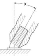
bend the welding element (1) with the bending device once by 30° in any direction.
