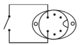
Pin 3; 4 is to be short circuited for at leasts 100 ms for the welding start.
