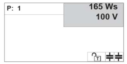
One or two capacitors are illustrated on the top right of the display:
